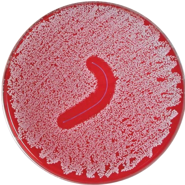
Shown: VICRYL* PLUS Antibacterial (polyglactin 910) Braided Suture creates a zone of inhibition to prevent Staphylococcus epidermidis bacterial colonization in sheep's blood medium.
